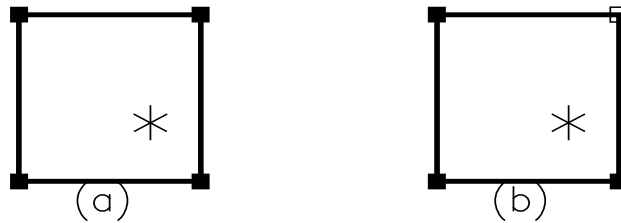
Figure 7.2. Location of the four points used in the interpolation of tidal data to a point (*). For the left rectangle (a), the four values are non-null (filled squares), so the bilinear interpolation method is used. For the right (b), since one of the values is null (open square), an inverse-distance-squared weighting method is used.
